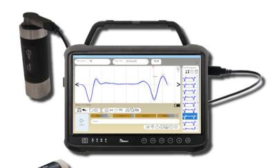
PET is used to test the integrity of deep pile foundations. PET Uses the pulse-echo method (PEM) for pile integrity testing (PIT).
